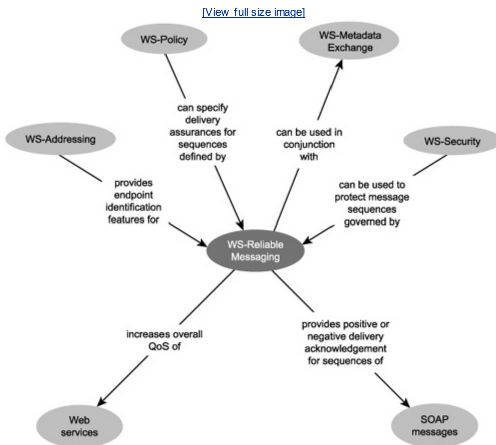
Figure 17.2. How WS-ReliableMessaging relates to the other WS-* specifications discussed in this chapter.
