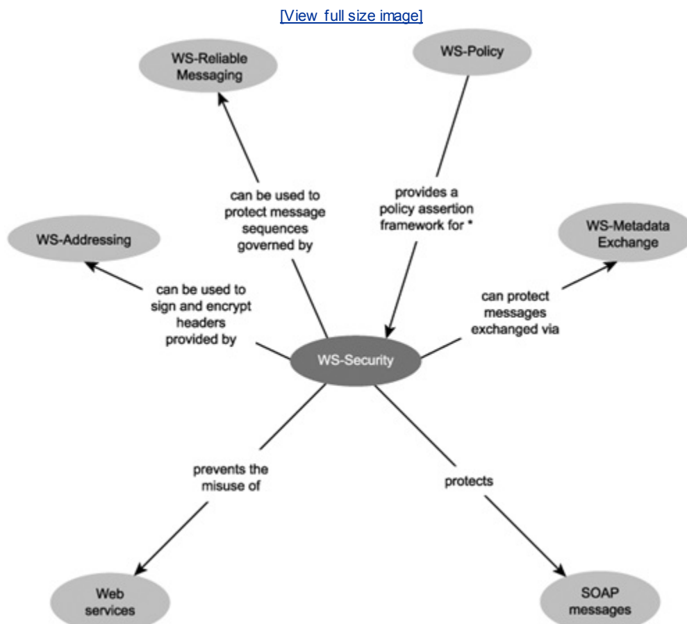
Figure 17.5. How WS-Security relates to the other WS-* specifications discussed in this chapter.
