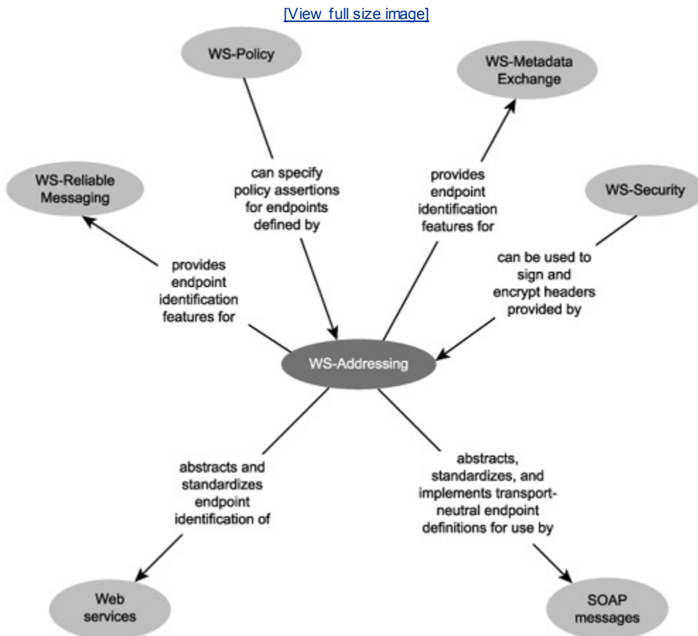
Figure 17.1. How WS-Addressing relates to the other WS-* specifications discussed in this chapter.
